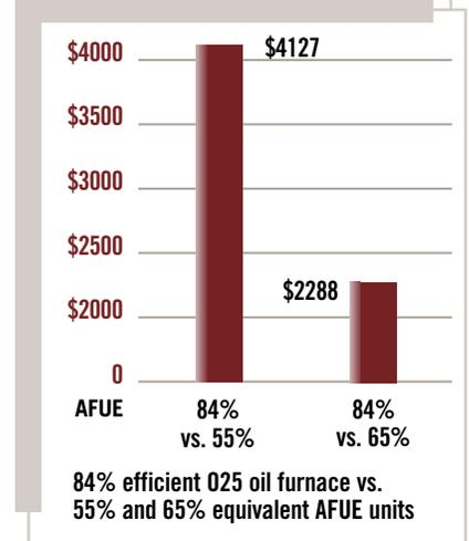
This chart depicts potential energy savings you can expect from the O25 furnace versus older furnaces with lower efficiency ratings. Criteria used in this example are 2,000 full-load heating hours, with a 80,000-Btuh heating design load and \$1.90 per gallon for oil. Your actual savings will vary depending on the weather, local fuel rates and your lifestyle.
