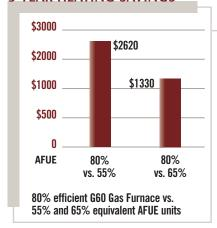
This chart depicts potential energy savings you can expect from the G60 gas furnace versus older furnaces with lower efficiency ratings. Criteria used in this example are 2,000 full-load heating hours, with a 60,000-Btuh heating design load and \$1.281 ccf for gas. Your actual savings will vary depending on the weather, local fuel rates and your lifestyle. Source: EPA national average energy rates.
